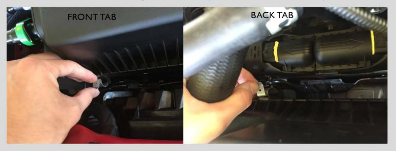
c. Lift airbox lid from left side (passenger side) to unfasten the lid from its locking hinges.
