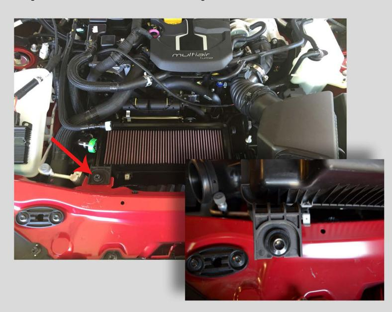
e. Once this is complete, wrap your hands around the base of the airbox, and the entire thing can be pulled out of the engine bay. The fresh air ducting attached to the bottom left side of the airbox will disconnect as you pull the airbox out.
