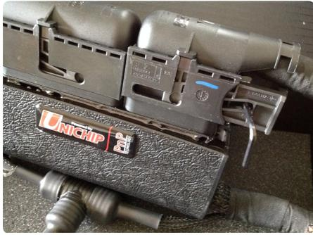
8. Slide is fully retracted and now you can disengage Unichip harness plug.
