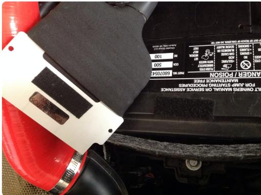
20. You can mount the booted Unichip on the battery by securing it with the supplied velcro. Or the Unichip can be velcroed to the back of the ECU (near the brake fluid reservoir).
