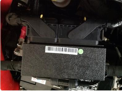
12. Repeat process to insert other stock harness plug into Unichip harness, again making sure plug sits snugly, level and securely before lowering lock arm. Relock yellow clip.
