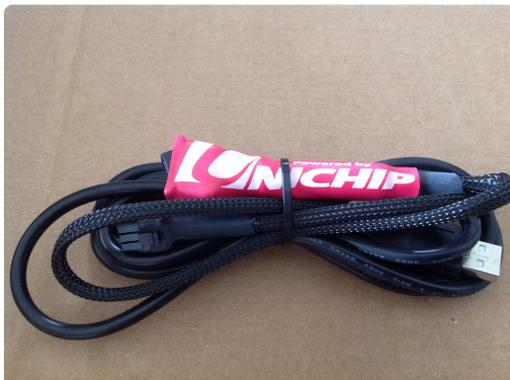
This is the interface USB cable you would use to upload Stage 2 or 3 to your Unichip through a PC or laptop.
