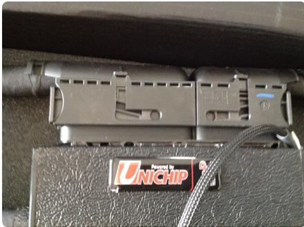
5. Next, you have to remove the Unichip plugs from the harness. This can be tricky as there are no yellow locking clips and no levers to lift to unlock plug slides and plugs are tight.
