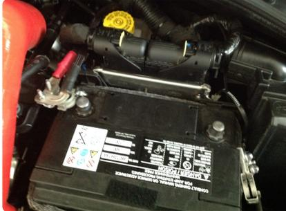
1. Disconnect battery both positive and negative terminals.
