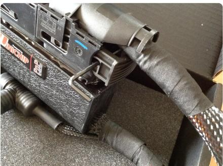
7. Insert a small enough in diameter allen wrench, punch or screwdriver into that slot and *\*slowly\** and *\*gently\** wedge slide back using the inserted tool as leverage until slide is completely retracted.
