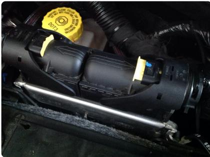
2. Disconnect stock ECU plugs from stock harness. Slide yellow locking clip first. Then, lift locking lever up all the way to disengage locking plug slide. (You will NOT be able to unplug both stock plugs at the same time, only one at a time)
