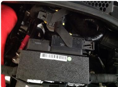
11. Insert stock ECU harness plug on Unichip harness, \*\*making sure harness sits snugly and nicely\*\* level before lowering arm to lock slide. Relock yellow clip.
