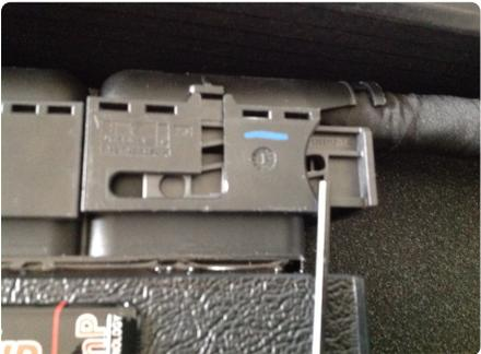
6. Pull slide back as much as you can, it will be tight. Look for the notch (where the allen wrench tip is pointing to).
