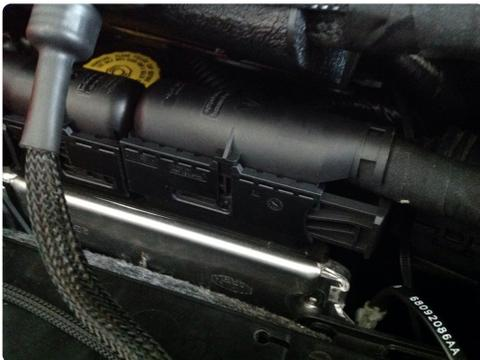
14. Repeat process to insert remaining Unichip harness plug into stock ECU. Push locking slide back in.
