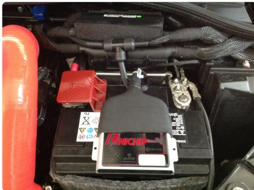
21. Finished look. Make sure to do a hard reset by disconnecting both battery terminals. Follow Unichip break-in procedure found on Eurocompulsion website and enjoy!
