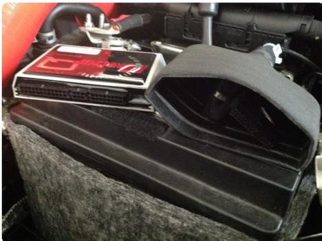
17. Take you Unichip and observe the orientation of the plug inside the rubber boot to make sure you plug it in correctly.
