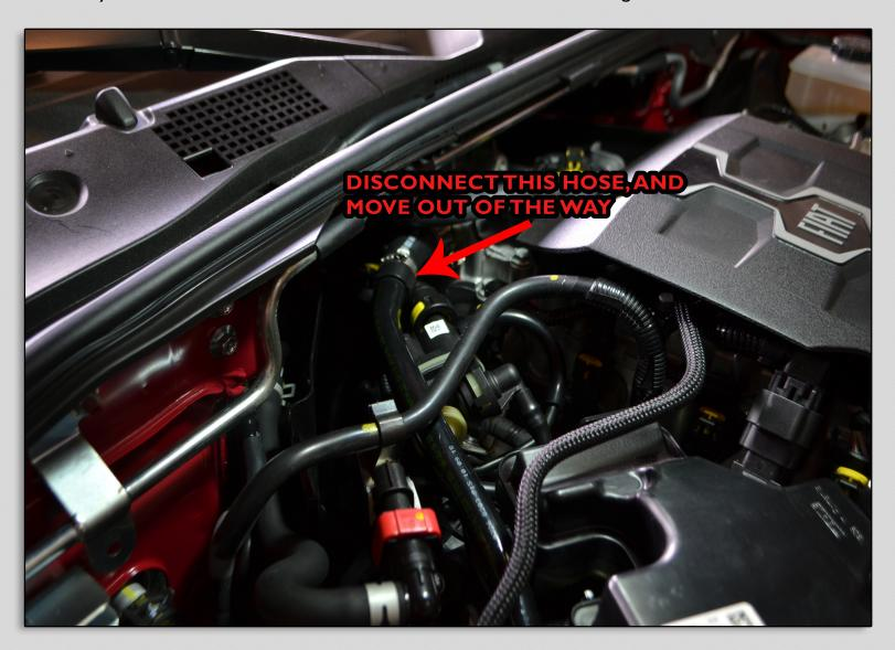
Once these two things are out of the way, you can fit your left hand behind the engine and disconnect the factory connector from the RPM sensor and connect the EDL connectors. You will have to do this entirely by feel, so it's tough. Expect to spend about 30 minuets struggling with this.
