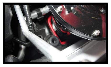
• Attach included 14mm breather hose to Apollo filter and fitting on engine block.
