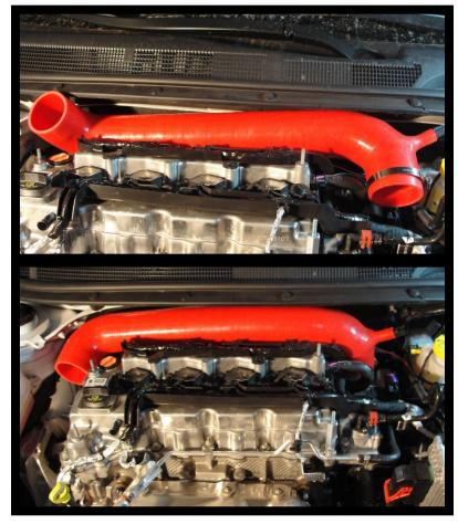
• Connect joiner to opening on tube. Place joiner mounting hose over stock engine cover stud. Be sure to put the shorter side of the joiner towards the back of the vehicle. It should be at an
