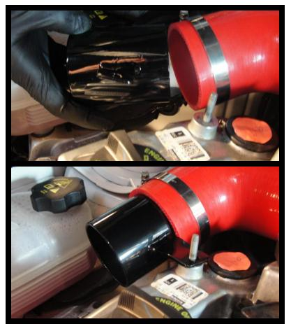
• Place included washer and nut on engine head stud. Hand tighten until the joiner is secured, **DO NOT use wrench to tighten it yet.**
