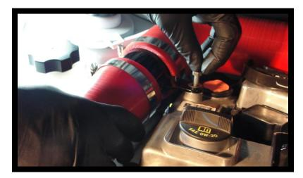
• If you removed the stock resonator in wheel well be sure to use included split silicone hose to line the inside of the air box mount.
