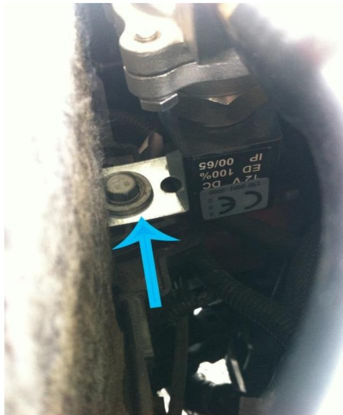
**\*\*The arrows drawn on the valve indicate direction of flow. In order for the valve to work properly with the hose routing, you should have the valve positioned and installed so that the arrows point towards the engine.\*\***
