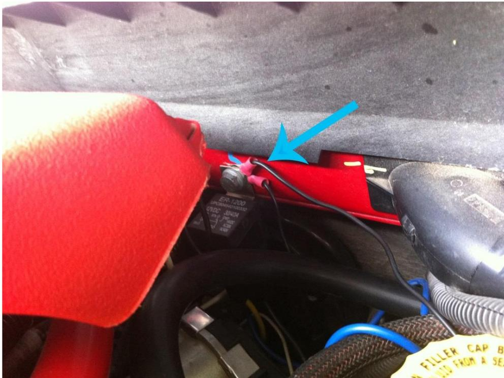
Next, we need to connect the two power wires. The first wire goes from the **valve** to the top terminal labeled “COM” on the **pressure switch** with a provided male connector. The second wire goes from the middle terminal on the pressure switch labeled “NO” to the battery positive terminal where it connects with a provided ring connector.
