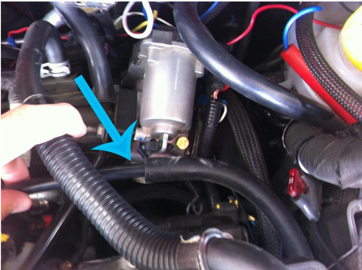
After you’ve made the cut, there are now two hoses: **1). The end of the hose coming from the boost pipe, and 2). The end of the hose going back to the air intake.**
