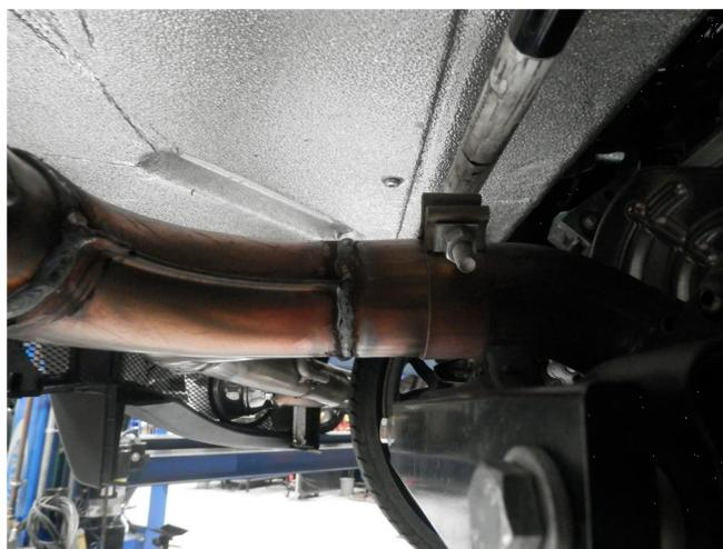
**Step 3.** Next loosely attach the Tail Pipe Assembly to the Inlet Pipe Assembly using the supplied 2.50" clamps. Engage all welded hangers to the rubber insulators.
