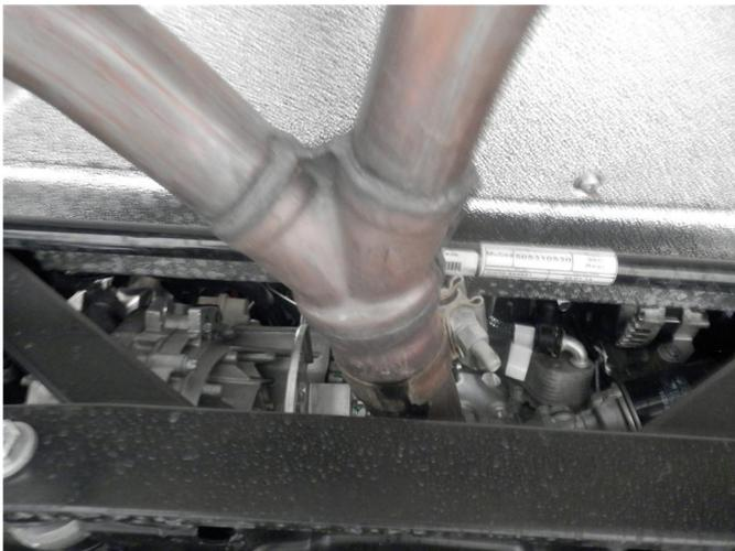
**Step 1.** To remove the OEM exhaust system you will need to loosen the band clamp attaching the Tail Pipe Assembly to the Inlet Pipe Assembly. Next Unbolt the Inlet Pipe Assembly at the flange junction. Remove the O2 sensor. Disengage all welded hangers from the rubber insulators and remove the assembly. Do not discard the or damage the rubber insulators as they will be used to mount the new system.
